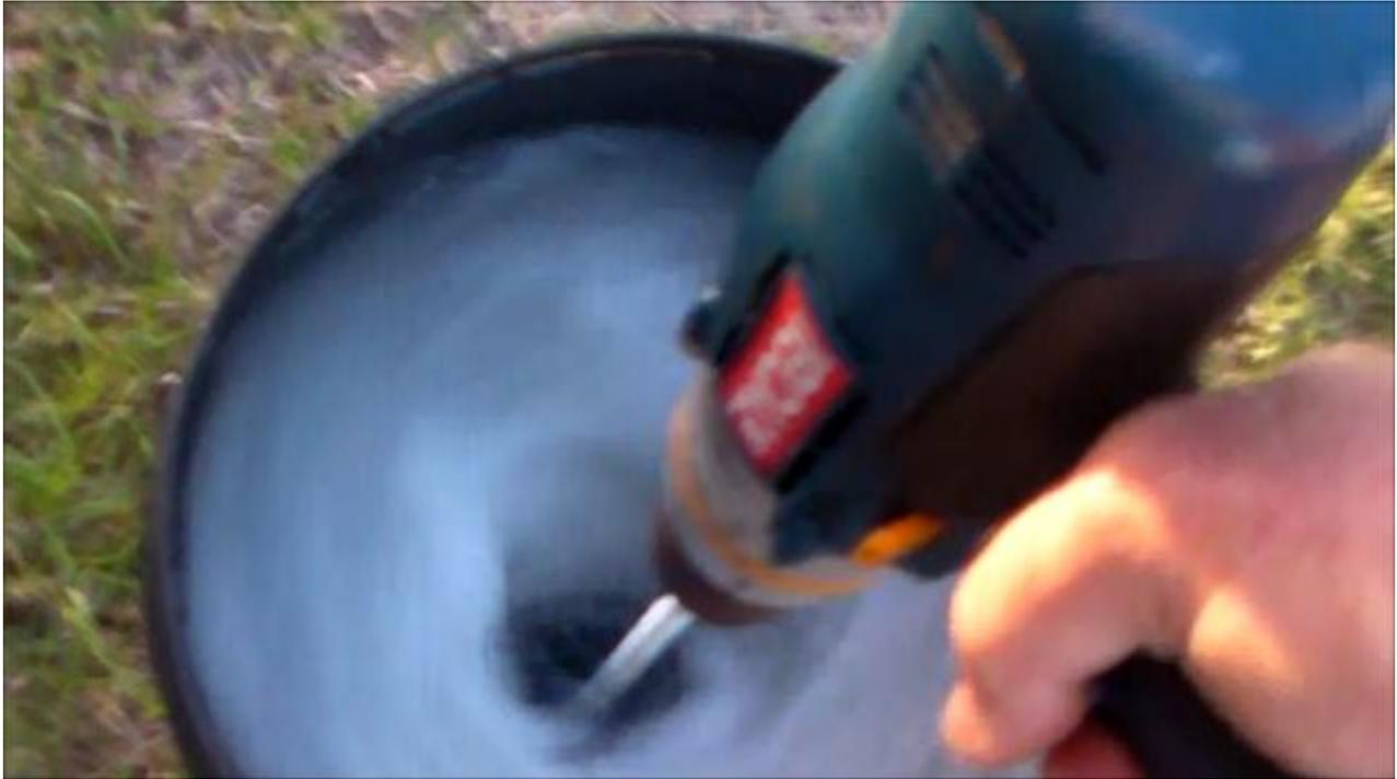
*Vortex Aeration at 300 RPM and 0.4 Watt*
